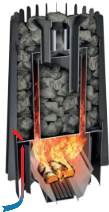
Fig. 3 Heater design and operation
