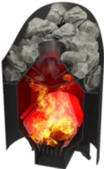
Fig. 4 Heater design and operation
